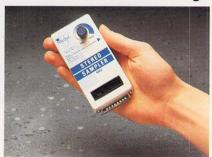
The latest version of Trilogic's sampler comes as a simple box equipped with a through-port for your printer, a stereo input and a gain dial. Also included is a simple beginner's piece of software and (gasp) an input lead!
